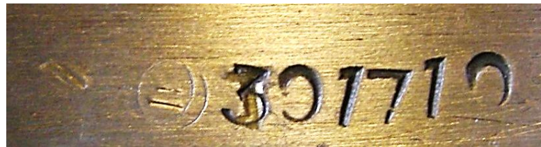
"He" of Heijo Factory, Jensen Army Arsenal with Clause 2 stamp (Alternate-spec weapon)
